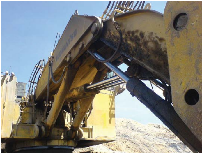
Figure 15 - Hydraulic cylinders blocked in open position at end of stroke.
