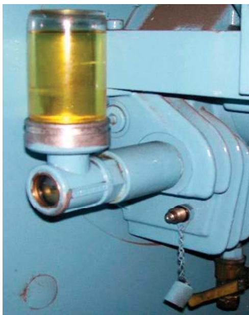
Figure 8 - A drop tube, through a reservoir wall or level check plugs allow for good representative samples.
