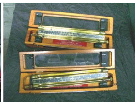
Figure 11 - A visgage for testing viscosity.
