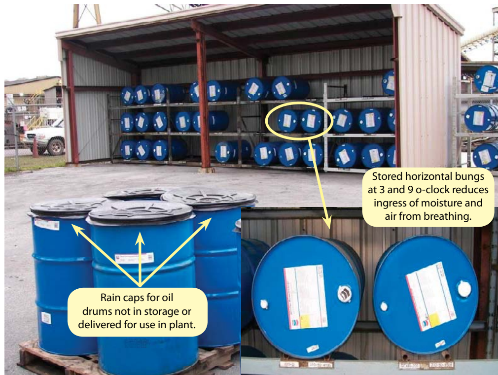
Figure 2 - Easy steps to take that will increase shelf life of lubricants by keeping contaminants at bay.
