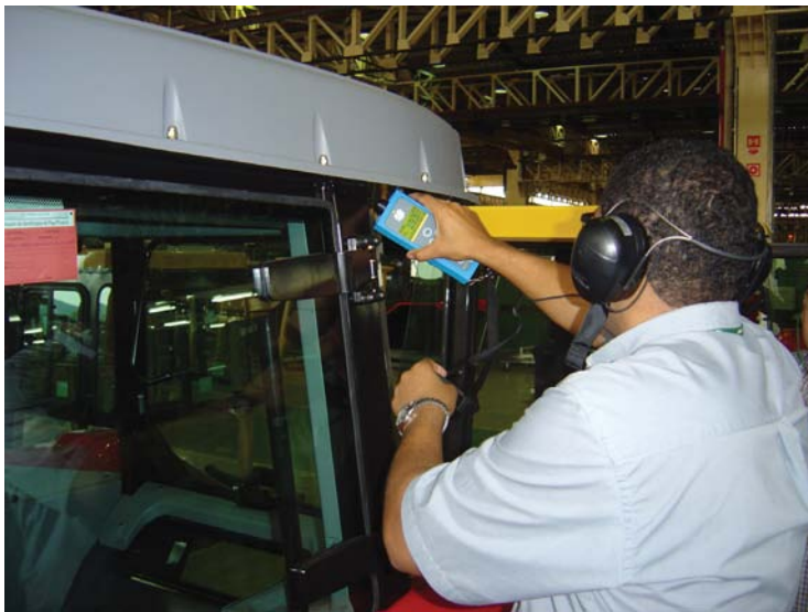
Figure 20 - Ultrasound inspector checks for tightness of tractor cab at SIAC do Brasil with his SDT170 and SDT08 ultrasound transmitter.
