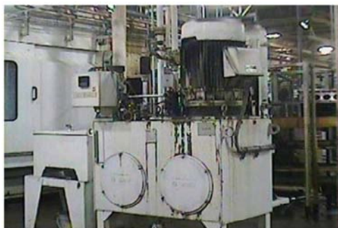
Figure 2 - IR camera thermograph (top) and visual photo (bottom) of an overheated hydraulic power unit reservoir.
