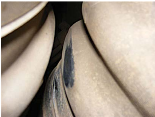
Figure 13 - Rubbing and leak discovered when pipes were pulled apart.
