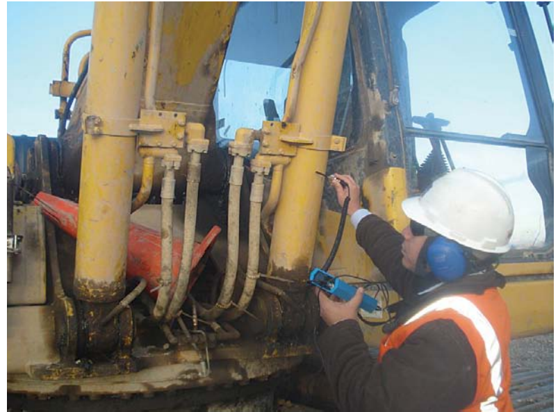
Figure 16 - Place sensor on barrel of cylinder near piston.
