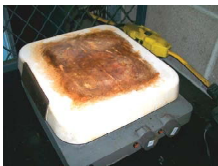
Figure 9 - A hot plate for water crackle test.
