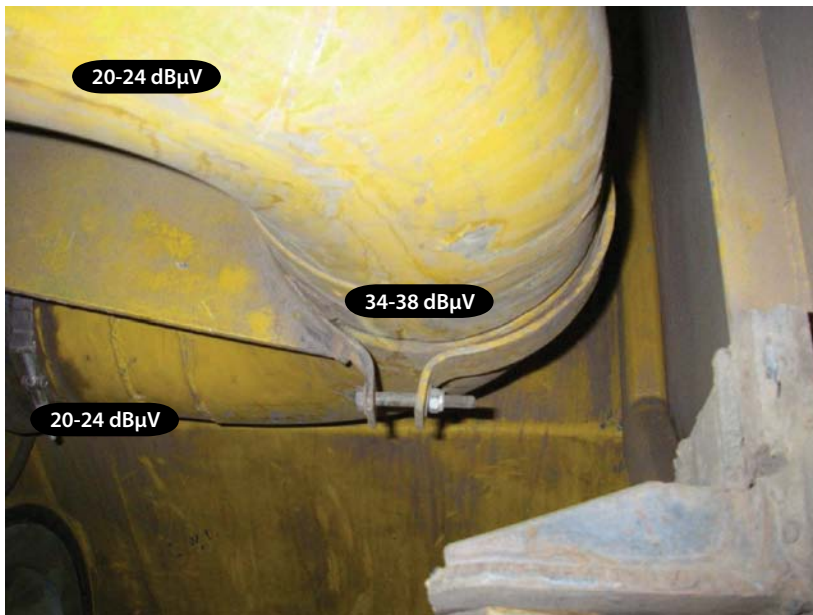
Figure 8 - The breather system was ultrasonically scanned from filters to turbo charger. One location was significantly higher than all others.
