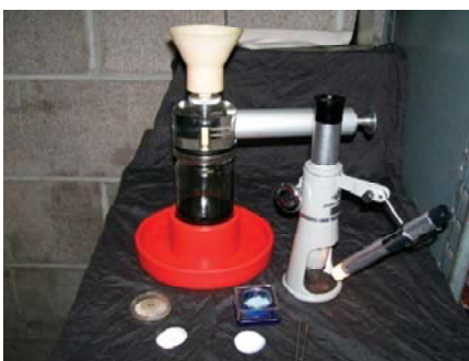
Figure 10 - A patch test kit.
