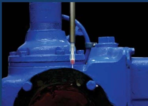
The Grease Thief with stinger probe shown in a motor operated valve application.
