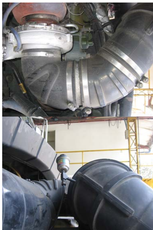
Figure 5 - Potential Leak Sites on piping between air breather and turbo charge
