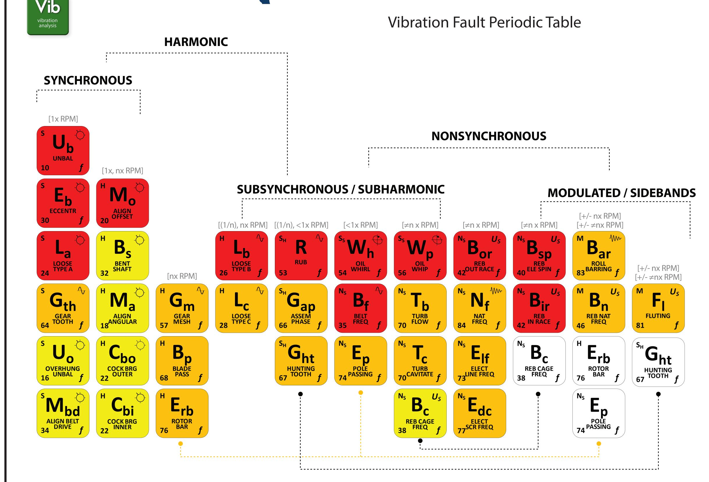
A logical visual mapping system to understand vibration analysis as "systems thinking." 1. Define the frequency grouping 2. Define the "dominant" directional response 3. Perform the recommended diagnostic test 4. Quickly narrow down the potential faults Frequency Grouping — Diagnostic Color / Directionality Formula Association Reference / Help **RADIAL AXIAL** RADIAL and/or AXIAL FREQUENCY GROUP **WAVEFORM PHASE**
